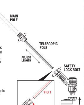
**WARNING: Bionic Trimmer** might not work for safety reason if the metal pole is not pushed all the way in.
