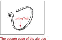
should face down, and the locking teeth should face up.
