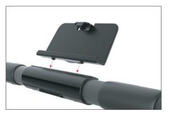
3 Using the screws provided, align the tablet with the holes on the upper part of the handle. Insert screws and tighten using the Allen key. Ensure the front lip is facing in the direction of the running belt for correct orientation.
