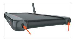
If the belt is not aligned, use the Allen key provided to loosen the bolts as located.
