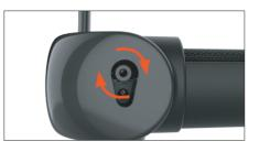
2 Once loose this will reduce the tension of the running belt and allow the belt to be realigned. Carefully move the belt in the required direction, making sure the belt is repositioned to be equidistant from each side.
